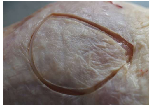
Fig. 5: This cut into the cutis of a chicken thigh was made with a single incision. The cut edges are smooth. The width of the coagulation zone at the cut edges can be adjusted to suit the purpose by making settings on the HF generator.
